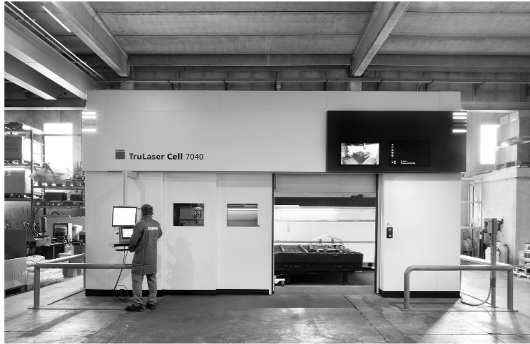
3d laser cut machine installed at the company.
